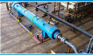
MAN Diesel & Turbo SE Renewal of piping circuit test bench, OB Piping of a compressor train consisting of a gas turbine and a compressor for testing on an open-air test bench. 3,750 hours September 2017 - March 2018
